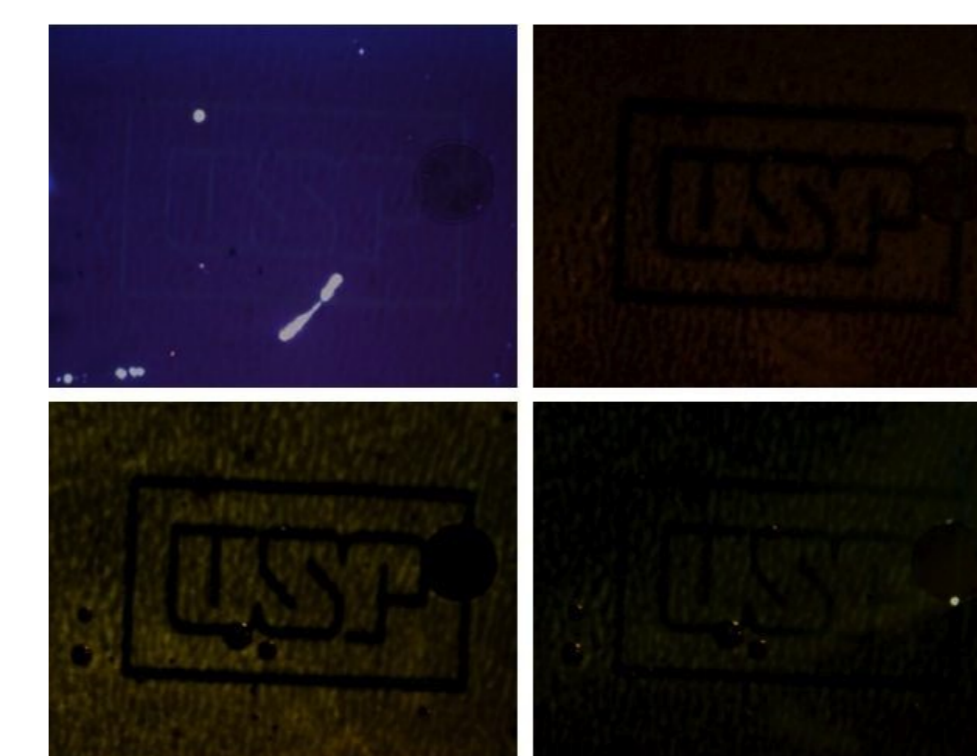
Images of the device of MEH-PPV (a) just before applying the voltage, (b) after 30 sec (c) is after 43 (d) after 55 s.
