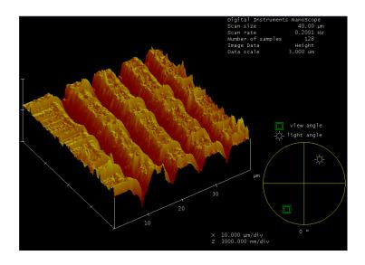
The depths of the grooves were determined using atomic force micrographs, and are plotted as a function of pulse energy. The groove depth increases with increasing pulse energy.
