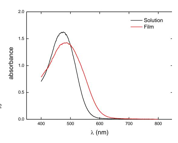
The UV-Vis absorption spectra of a chloroform solution (black) and film (red)
