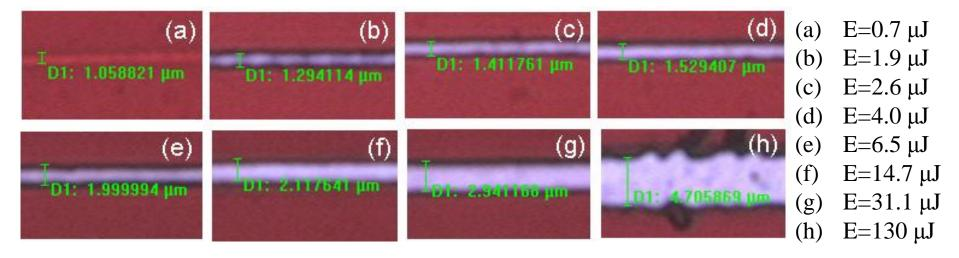
This figure shows optical microscope images of grooves produced on the sample at a translation speed of 1 mm/s and various pulse energies. The widths of the grooves vary from 1 to  $4.7~\mu m$  when the pulse energy is increased from 0.7 to  $130~\mu J$ .
