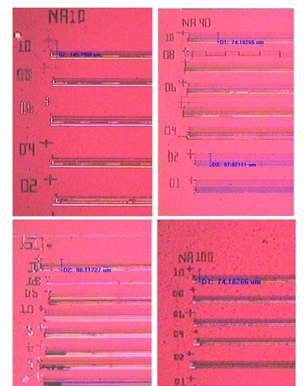
The influence of pulse energy and translation speed on the micromachining was studied using optical and atomic force microscopy.
