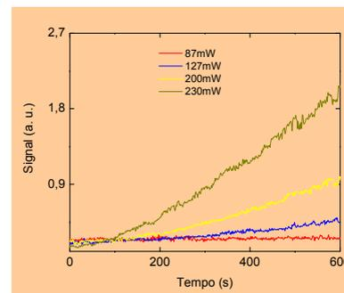
The quadratic dependence of  $\Delta n$  as a function of Irradiance corroborates the 2PA origin of the process.
