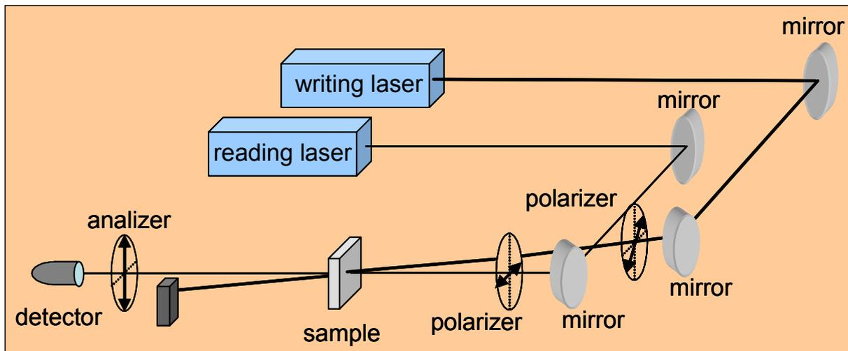
The 2PA birefringence was induced in the spincoated films using the linearly polarized 150 fs pulses at 680 and 775 nm (writing beam), delivered by the laser system used in the Z-scan measurements. The polarization angle of the writing beam was set at  $45^\circ$  with respect to the linear polarization orientation of the probe beam (reading beam). As the reading beam we used a low-power He-Ne laser at 632.8 nm passing through crossed polarizers.
