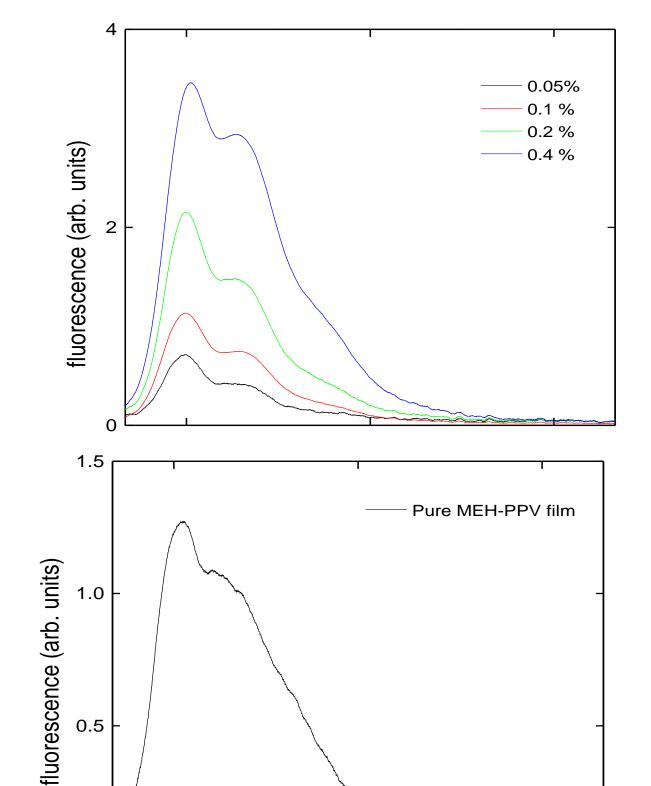
This figure shows the fluorescence spectra of thin films prepared with pure MEH-PPV and the polymeric blend with the acrylate resin. For excitation we used an Ar ion laser operating at 514 nm.
