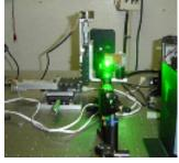
The picture shows the translation stages, the step motor coupled to micrometer and the laser beam focussed at the sample. The resolution of our system is ~4.8  $\mu m$ , nevertheless, the thickness of the tracks is defined by the spot size of the focussed laser heam
