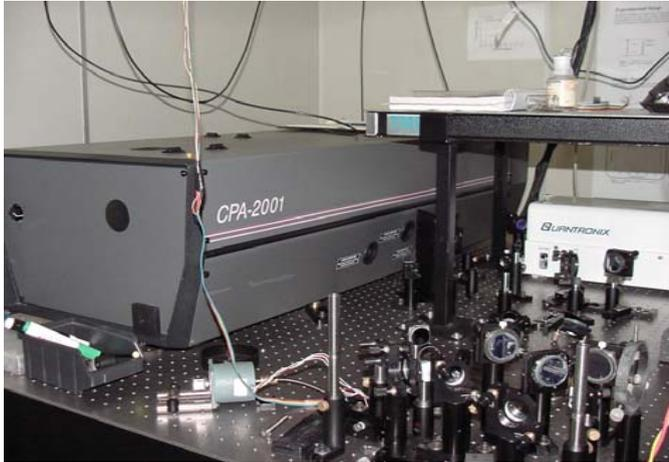
✓ *Ti:sapphire chirped pulse amplified system (CPA-2001)*
