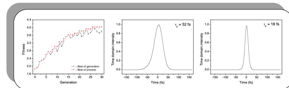
Figure 8: Evolution of the fitness parameter and the FROG measurements of the pulse before and after the optimization process via 2PEF.
