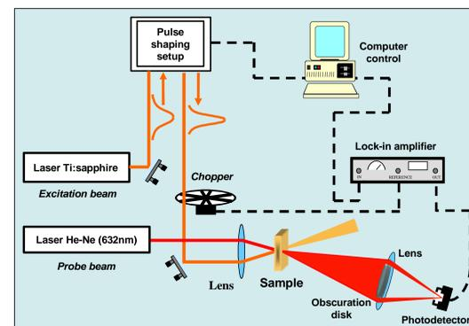
Figure 6: Experimental setup for pulse optimization via two-photon induced thermal lens.
