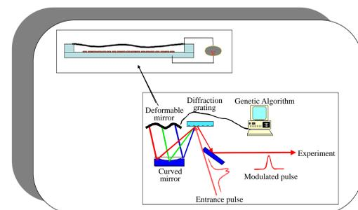
Figure 4: Experimental setup for pulse shaping.
