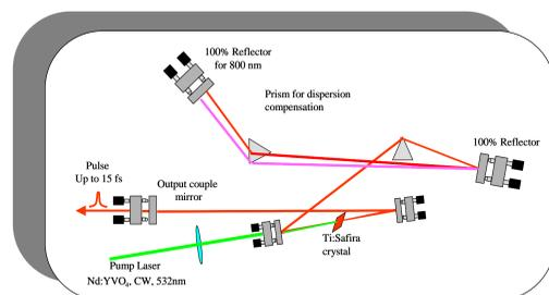
Figure 3: KLM Ti:sapphire femtosecond laser cavity.
