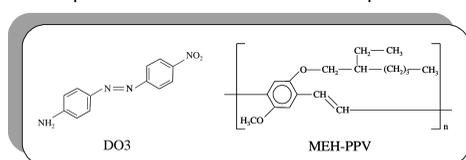
Figure 1: Molecular structures of the compounds employed.
