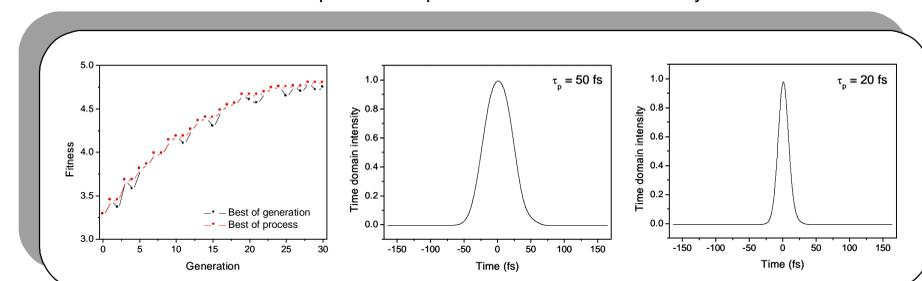
Figure 7: Evolution of the fitness parameter and the FROG measurements of the pulse before and after the optimization process via 2PTL.
