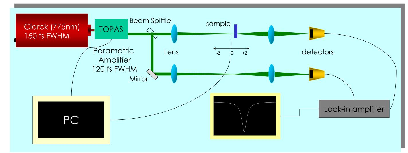
Our Z-scan experiment employs laser pulses from a commercial optical parametric amplifier (TOPAS) pumped by a 150 fs pulses at 775 nm delivered by a Ti:sapphire chirped pulse amplified system (CPA-2001, from Clark-MXR Inc.), operating at 1kHz repetition rate.
