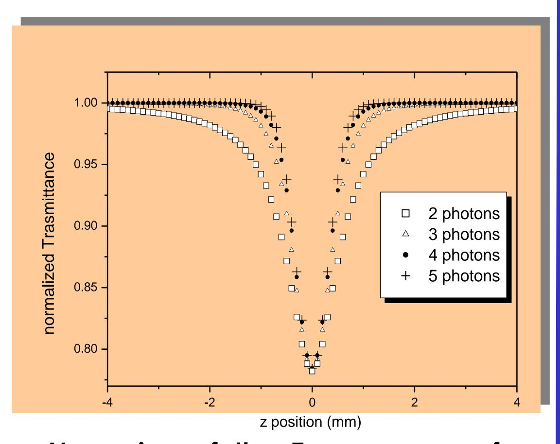
Narrowing of the Z-scan curves for higher values of n due the need of a higher pump intensity
