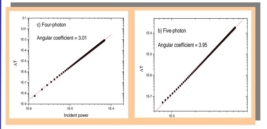
The simulated curves for normalized transmittance change ( $\Delta T$ ) as a function of the excitation beam showed different slopes for the two-, three-, four-, and five-photon absorption processes .
