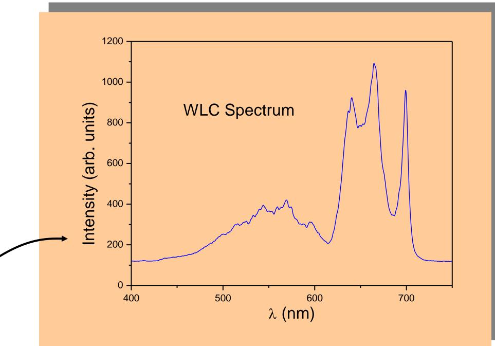
Using about 0.1 mJ of 150 fs Ti:sapphire laser pulse we were able to generate about 3  $\mu$ J of WLC in the visible range using the 4 cm length water cell. An IR filter was used to remove the strong 775 nm pump pulse. This spectrum is a function of the intensity and the wavelength that is applied in the water cell.
