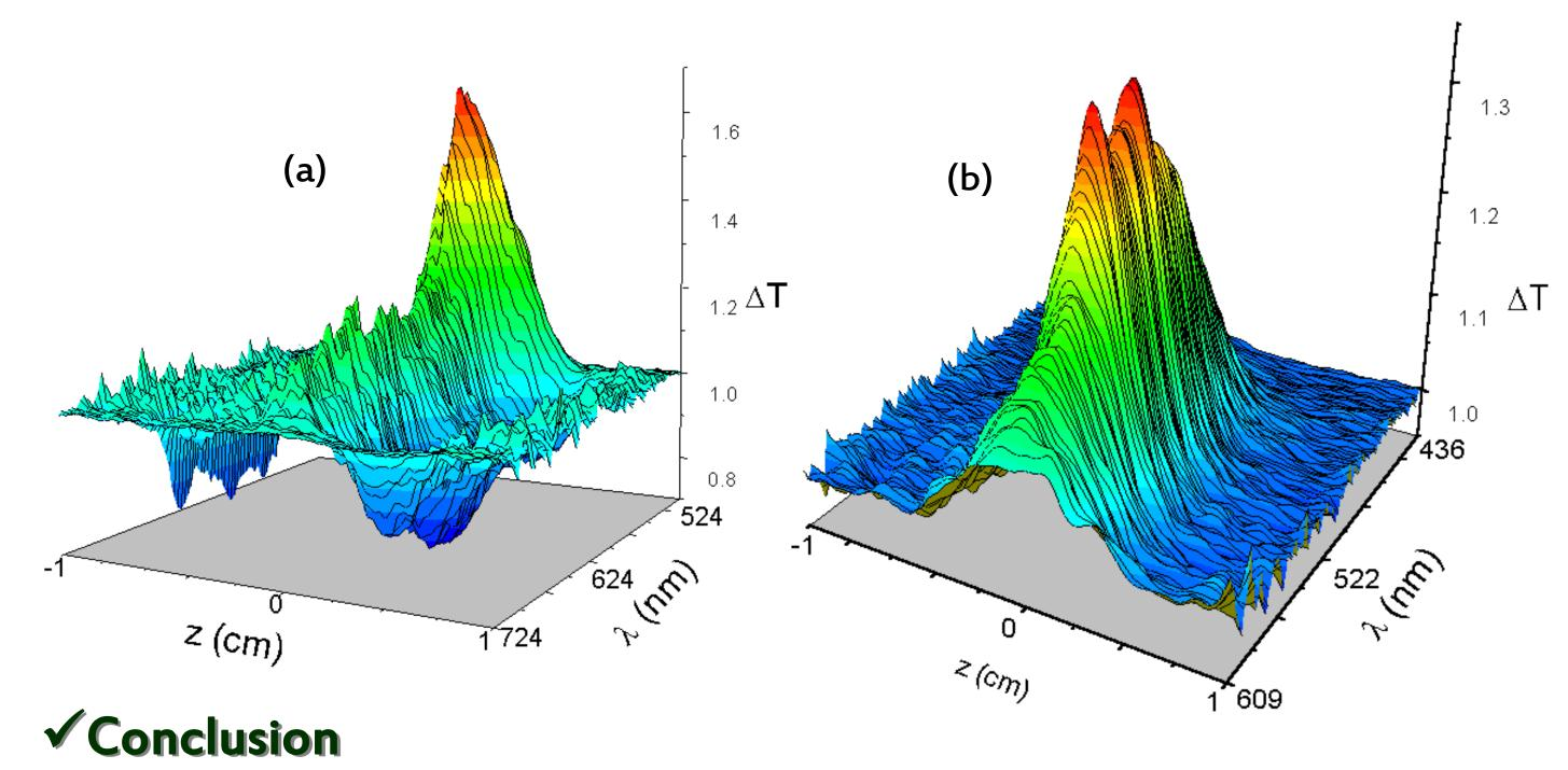
In summary, we have demonstrated a new experimental method for measuring the nonlinear absorption spectra in a single measurement using white-light continuum beam. A good agreement between the results obtained by the method using a WLC and the traditional discreet measurements. These results allow concluding that the Z-scan
