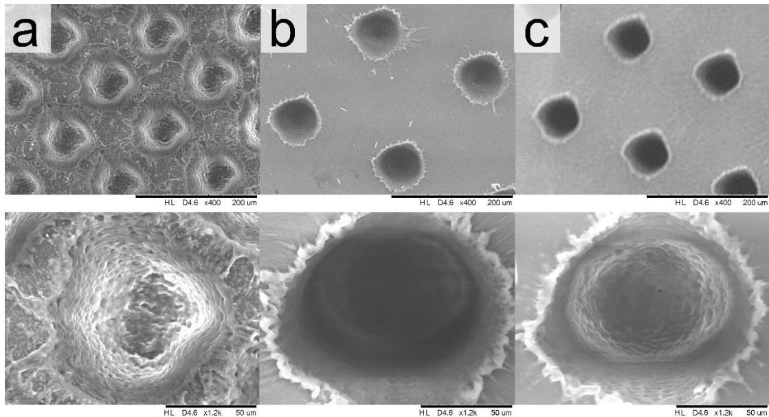
SEM images of micropores created with (a) 35 pulses/pore ( $8000 \text{ pores/cm}^2$ ) and no nitrogen flow. (b) and (c) 50 and 100 pulses/pore respectively ( $4000 \text{ pores/cm}^2$ ) and constant nitrogen flow.
